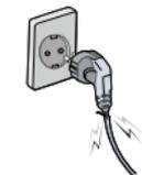
If a power plug is broken or a plug is cut or worn, do not use it.
