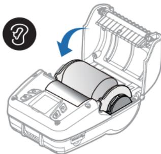
Pull a short length of paper out of the printer and close the cover.
