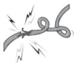
**Do not bend the wire and do not allow the wire to be pinched or crushed by heavy objects.**
